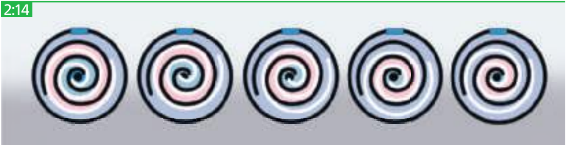
Compression principle of a scroll compressor.
